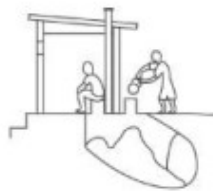
Composting latrine — needs careful operation and separate urine collection. However, composting toilet systems and other similar wastewater management methods — where waste is turned into humus — are increasingly considered the ecological alternative; see Del Porto and Steinfeld, 2000.
