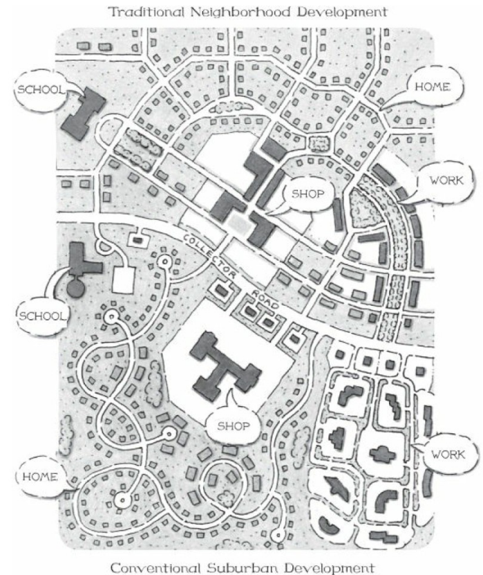
Figure 15.4 Schematic Comparison of Street Networks and Land Use in a Traditional Neighborhood and in an Area of Sprawl
